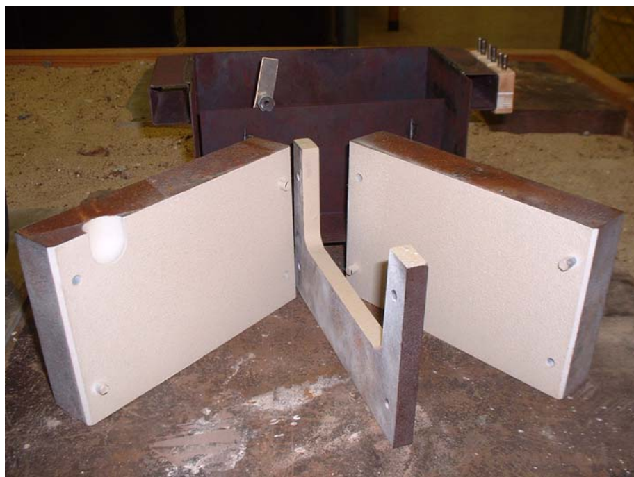
Figure 3.1 - Three-piece Steel Mold (disassembled)
