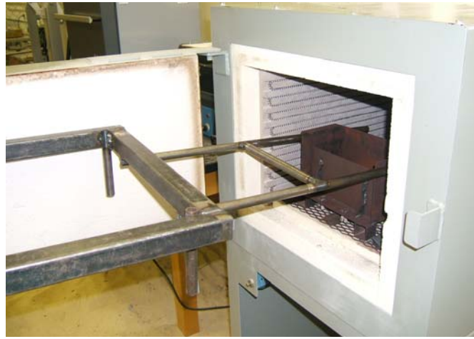
Figure 3.14 - Mold Carrier Removal Process (staged)
