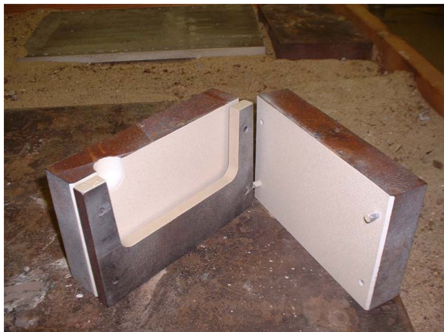
Figure 3.2 - Three-piece Steel Mold (partially assembled)
